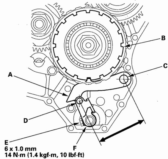
27. If the park pawl does not engage fully, check the distance between the pawl shaft (C) and the park lever roller pin (D) (see page 14-254).
