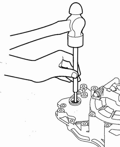
2. Install the new bearing flush to the end cover with the special tools.
