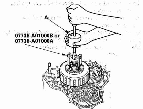
15. Remove the splined washer, thrust needle bearing, countershaft 3rd gear, needle bearing, and thrust needle bearing from the countershaft.
