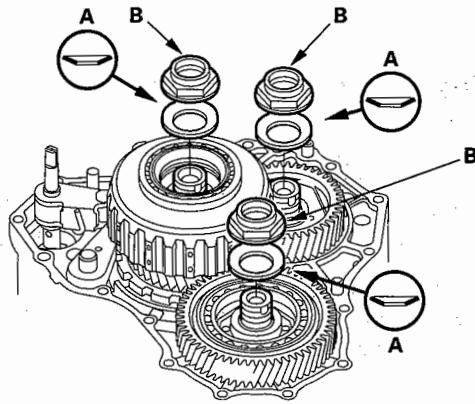
23. Tighten the locknuts to 167 N·m (17.0 kgf·m, 123 lbf·ft).
