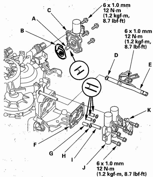
34. Install the new gasket (B) in the mounting groove of the A/T clutch pressure control solenoid valve C body (C) properly, then install them on the transmission housing. Do not pinch the gasket.
