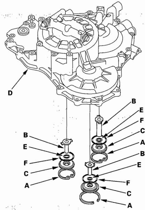
2. Install the new O-ring (E) over the ATF feed pipe.
