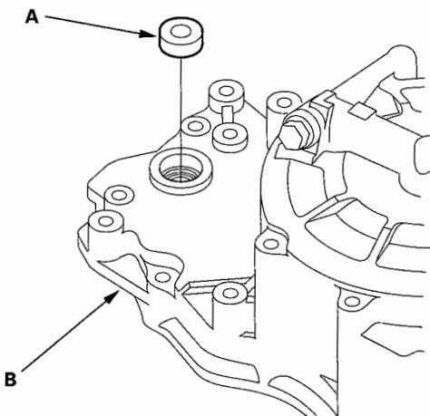
2. Install the new oil seal flush to the end cover with the special tools.
