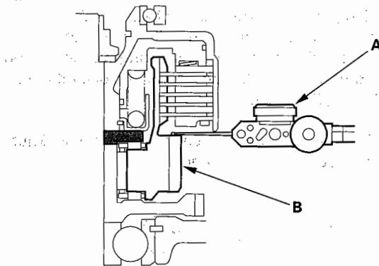
7. Measure the countershaft 3rd gear axial clearance in at least three places, while moving the countershaft 3rd gear (A). Use the average as the actual clearance.
