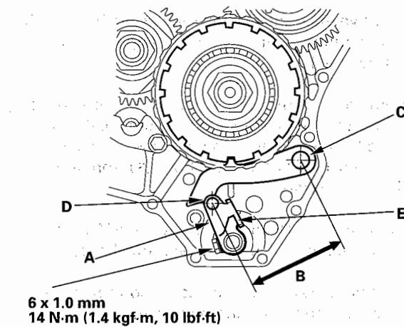
2. Measure the distance (B) between the park pawl shaft (C) and the park lever roller pin (D).
