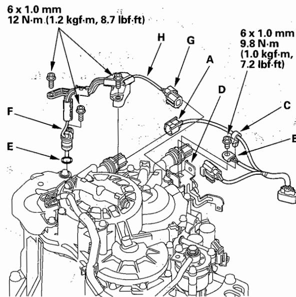
50. Install the new O-ring (E) on the ATF temperature sensor (F), then install the sensor in the end cover.
