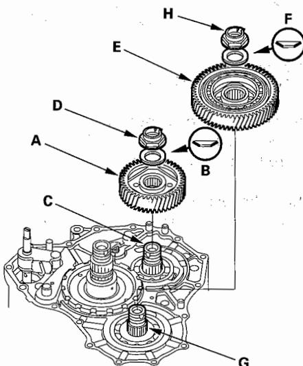
14. Install the secondary shaft idler gear (E) and the old conical spring washer (F) on the secondary shaft (G). Tighten the old locknut (H) to seat the secondary shaft idler gear to 226 N·m (23.0 kgf·m, 166 lbf·ft).
