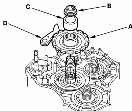
4. Remove the locknut and collar.
