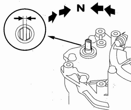
44. Align the cutouts (A) on the rotary-frame with the neutral positioning cutouts (B) on the transmission range switch (C), then put a 2.0 mm (0.08 in.) feeler gauge blade (D) in the cutouts to hold the switch in the N position.
