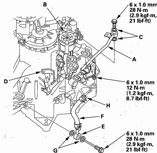
41. Install the ATF line (E) and hose (F) on the torque converter housing with the line bolt and new sealing washers (G).
