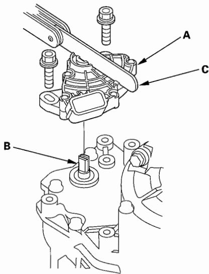
46. Tighten the bolts on the transmission range switch while you continue to hold it in the N position. Do not move the transmission range switch when tightening the bolts. Remove the feeler gauge.
