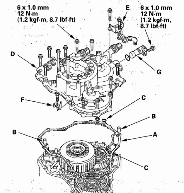
30. Install the end cover (D), and install the 16 bolts, connector bracket (E) and harness holder bracket (F).
