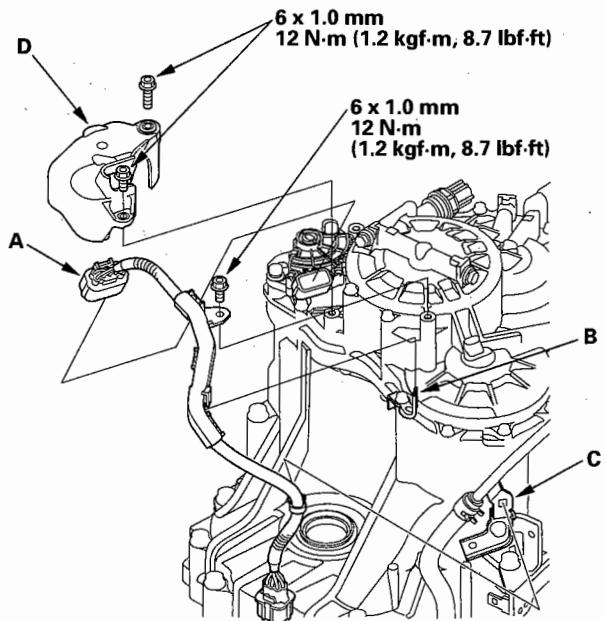
48. Install the transmission range switch cover (D).
