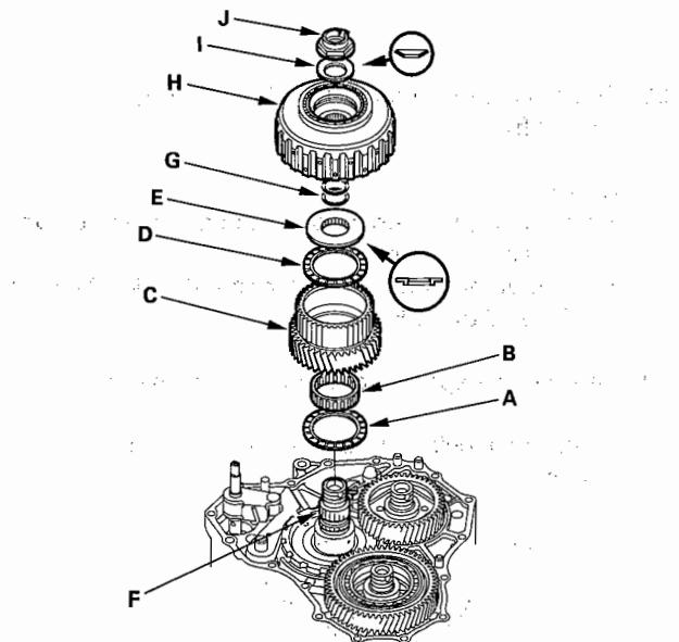
18. Wrap the shaft splines with tape to prevent O-ring damage, then install new O-rings (G).
