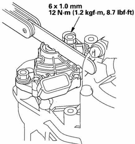
47. Connect the transmission range switch connector (A) securely, then secure the switch harness on the end cover, harness cover bracket (B), and the clamp bracket (C).
